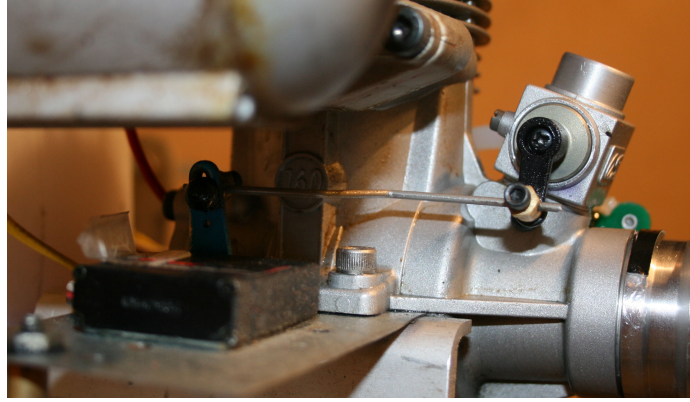
Figure 3.5: Servo and throttle arm linkage.
